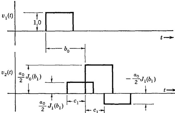
Fig. 4-37 "Paired echoes" resulting from phase distortion.
