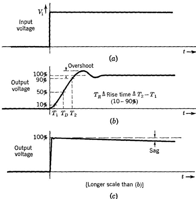
Fig. 1-4 Lowpass amplifier response to a step voltage input.
