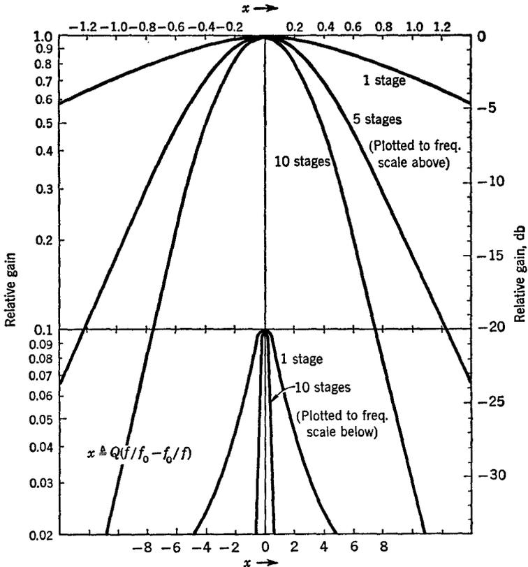
Fig. 7-5 Normalized gain-frequency curves for single-tuned interstages.
