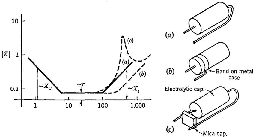
**Fig. 15-2** Impedance of a typical capacitor over a wide frequency range. (a) Impedance measured between the lead ends. (b) Impedance measured between lead and (metallic) case. (c) Effect of paralleling capacitors.
