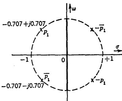
Fig. 9-4 Pole positions for  $n = 2$ , maximally flat function.
