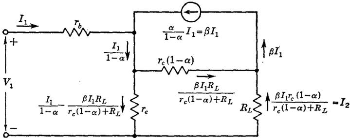
Fig. 3-16 Approximate currents in a common-emitter (CE) amplifier.
