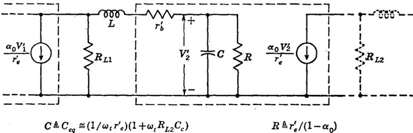
Fig. 4-13 Transistor equivalent circuit and series-peaked interstage.
