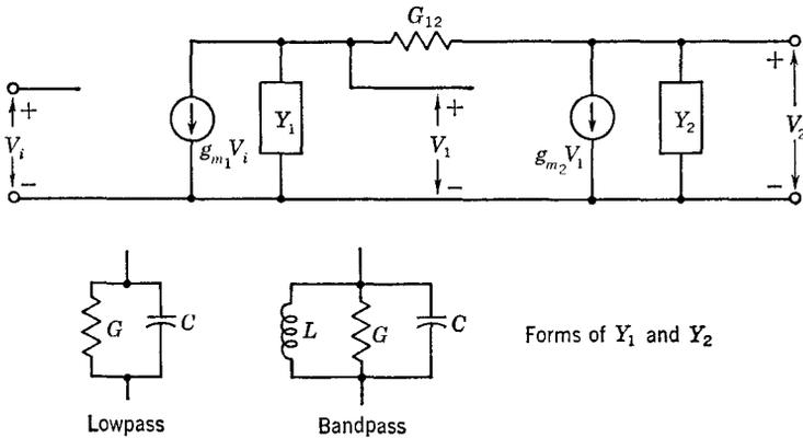
Fig. 12-1 Basic circuit of the feedback pair.
