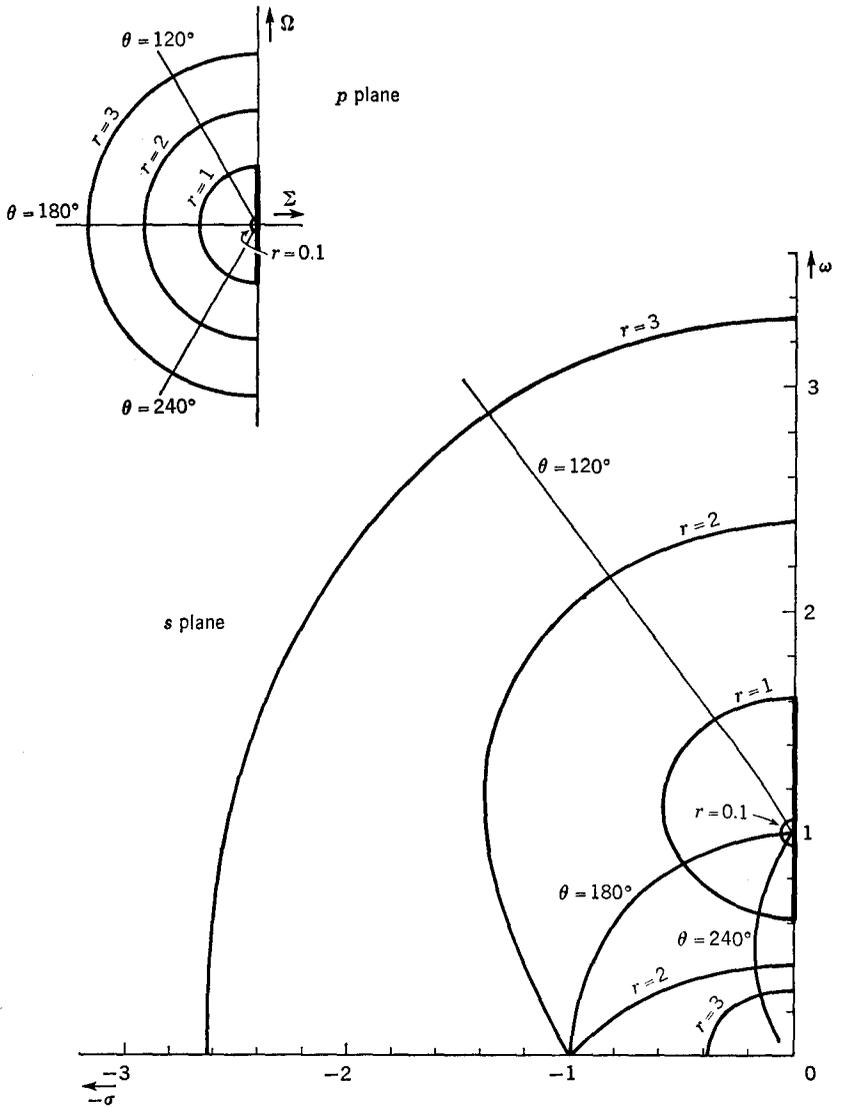
**Fig. 9-9** Transformation of pole loci from the  $p$  plane to the  $s$  plane by the transformation  $p = s + 1/s$ . The heavy line in the  $s$  plane shows the bandwidth which corresponds to the bandwidth (heavy line) in the  $p$  plane. Note that the heavy line in the  $p$  plane is twice as long as that in the  $s$  plane.
