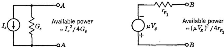
Fig. 14-7 Available powers in the circuit of Fig. 14-6.
