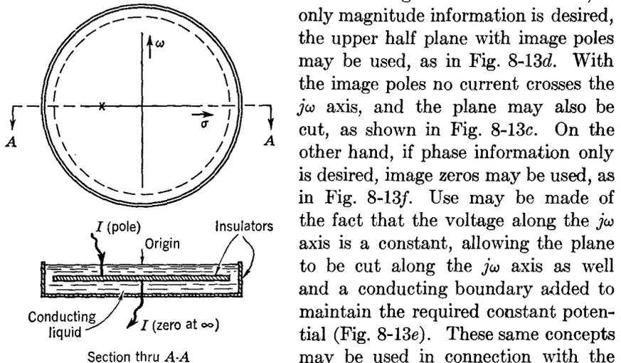
**Fig. 8-14** A method of eliminating the errors due to finite tank size in the conduction analogy. The conducting medium here is an electrolyte of uniform depth. The conducting path is folded under at the edge, and the point of infinity lies directly beneath the origin.
