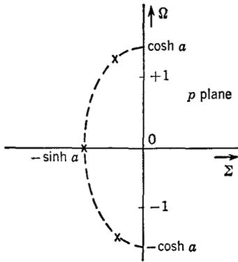
Fig. 9-12 Pole locations for an equal-ripple gain function.
