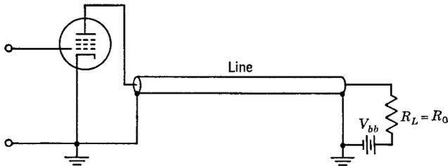
Fig. 4-30 A grounded-cathode amplifier driving a line.
