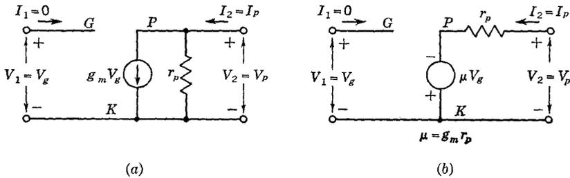
Fig. 2-4 Alternative equivalent circuits for pentode or triode.
