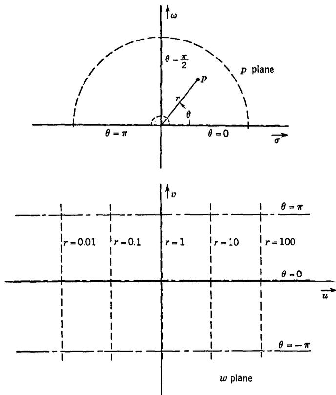
**Fig. 8-8** Illustration of the transformation  $w = \ln p$ .
