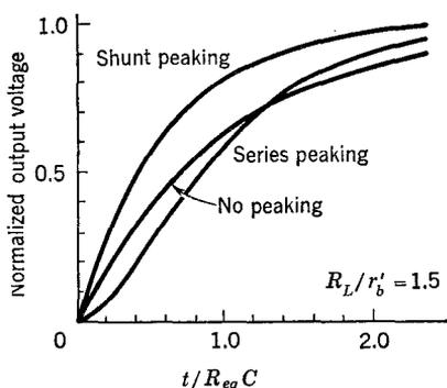
Fig. 4-21 Step response of a transistor stage.
