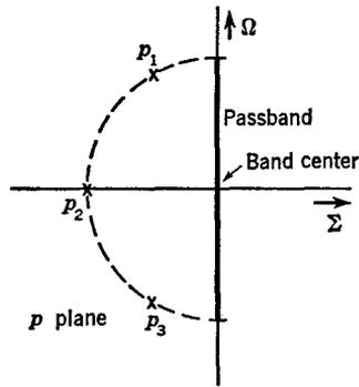
Fig. 9-8 Poles from Fig. 9-7 transformed to lowpass  $p$  plane.
