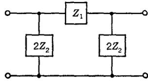
Fig. 6-6 Constant- $k$  prototype pi section.
