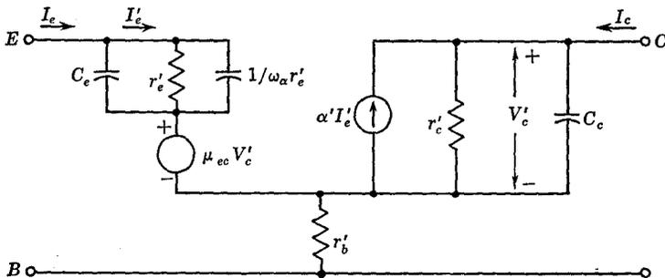
Fig. 2-19 The T equivalent circuit for high frequencies.
