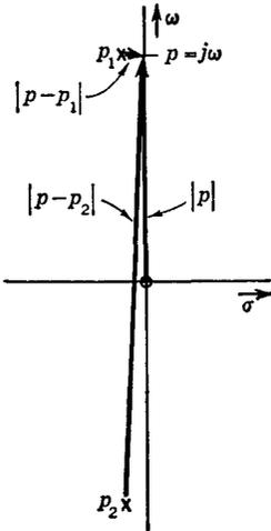
Fig. 8-2 Pole locations for a narrow-band stage.
