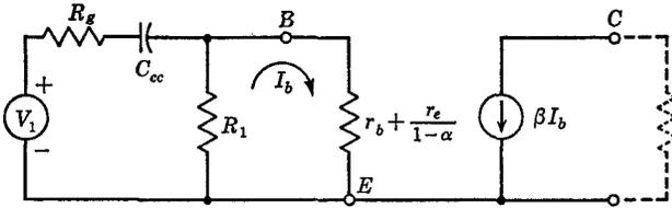
Fig. 3-33 Circuit for calculating the low-frequency cutoff due to the coupling circuit.
