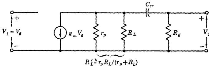
Fig. 3-4 Simplified circuit for determining the low-frequency gain.
