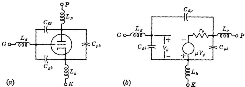
Fig. 2-14 Triode h-f equivalent circuits.
