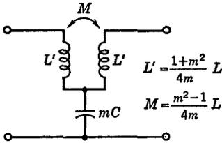
Fig. 6-13 Section using mutual inductance to realize  $m > 1$ .
