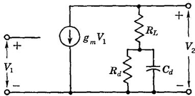
Fig. 5-7 Equivalent circuit for the sag-compensating circuit.
