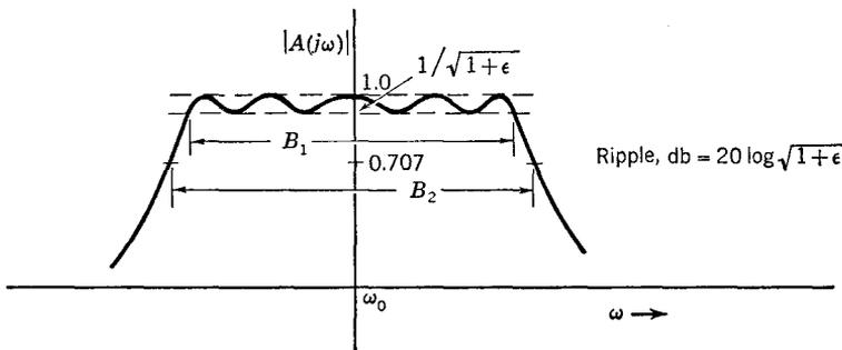
Fig. 9-10 Equal-ripple response.
