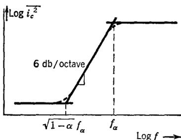
Fig. 13-5 Frequency dependence of the collector noise generator.
