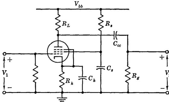
Fig. 3-27 A complete pentode stage for low-frequency analysis.
