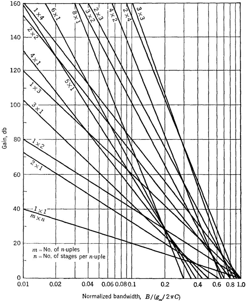
**Fig. 10-9** Gain-bandwidth chart for single-tuned stages. ( $n$ -uples are maximally flat.) [From B. A. Wightman, *A Graphical Method for Determining the Number and Order ( $n$ ) of  $n$ -uples in Stagger Tuned Amplifier Design*, Natl. Research Council Can., Rept. ERA-212, December, 1951.]
