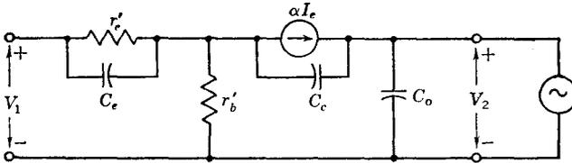
Fig. 15-16 The measurement of high-frequency  $h_{12b}$ .
