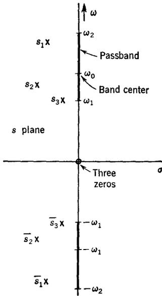
Fig. 9-7 Pole locations for a wideband triple.
