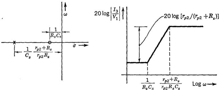
Fig. 3-35 Response due to the screen circuit alone.
