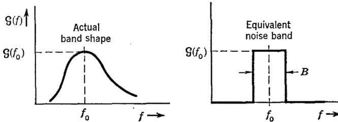
Fig. 14-5 The meaning of equivalent noise bandwidth.
