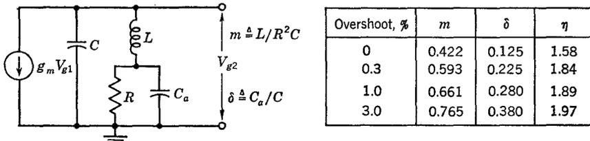
Fig. 4-5 An improved two-terminal network.
