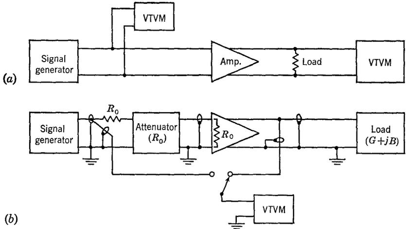
Fig. 15-17 Two methods of measuring amplifier gain.
