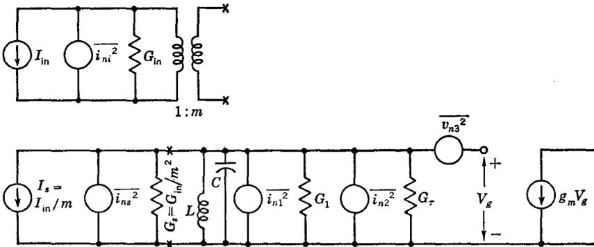
**Fig. 13-7** Equivalent circuit of the input stage of a vacuum-tube amplifier. [Adapted from G. E. Valley, Jr., and H. Wallman (eds.), “Vacuum Tube Amplifiers” (vol. 18, M.I.T. Radiation Laboratory Series), pp. 682–694, McGraw-Hill Book Company, Inc., New York, 1948; and M. T. Lebenbaum, *Design Factors in Low-noise-figure Input Circuits*, Proc. IRE, vol. 38, pp. 75–80, January, 1950.]
