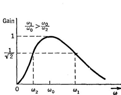
Fig. 11-14 Response of a double-tuned capacitively coupled interstage.
