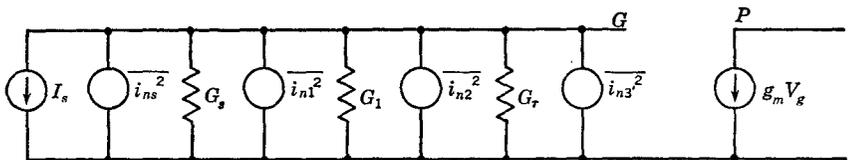
Fig. 13-9 Equivalent circuit for the calculation of  $F$ .
