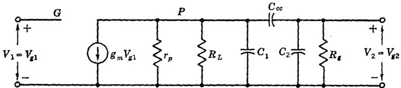
Fig. 3-3 Complete pentode equivalent circuit (omitting bias impedances).
