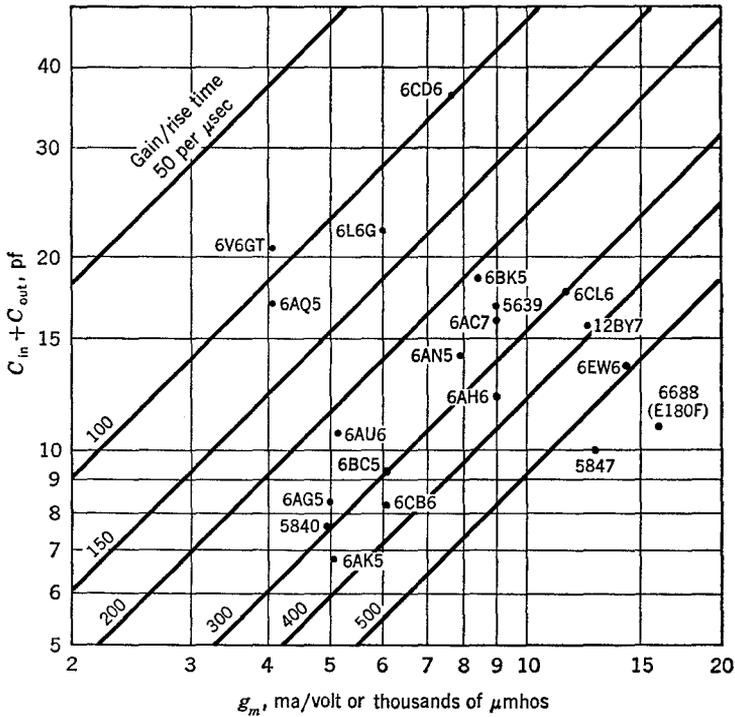
**Fig. 4-1** Comparison of tube types for gain/rise time. No allowance has been made for wiring capacitance; so any point should be moved vertically by the proper amount. Note that points for low- $C$  tubes move farther vertically for a given added wiring capacitance. Graphical presentation suggested by a similar plot from J. R. Whyte, *Electronics*, April, 1952.
