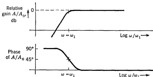
Fig. 3-5 Magnitude and phase of the gain of the circuit shown in Fig. 3-4.
