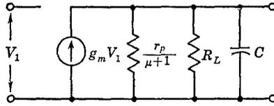
Fig. 4-31 An equivalent circuit for small-signal cathode-follower operation.
