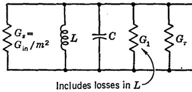
Fig. 13-8 Circuit for computing the input bandwidth.
