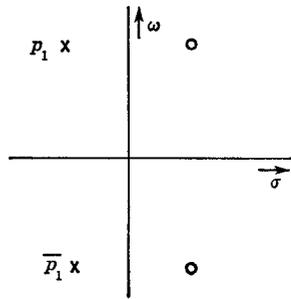
Fig. 9-17 Assumed pole locations of  $A(p)$  to give maximally flat delay.
