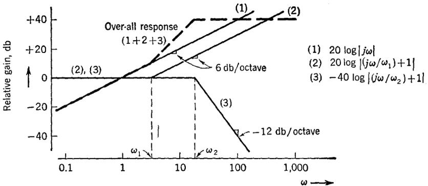
Fig. 3-8 Obtaining the amplitude response of Eq. (3-8c).
