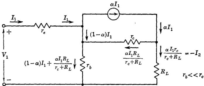
Fig. 3-15 Approximate currents in a common-base (CB) amplifier.
