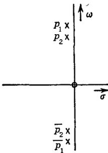
Fig. 11-2 Pole positions for the interstages of Fig. 11-1.
