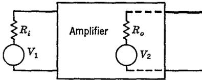
**Fig. 14-2** Circuit for definition of available power gain.
