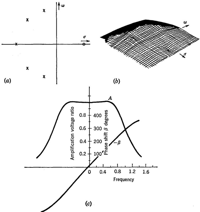
**Fig. 8-7** (a) Lowpass pole positions to give an approximation to both constant gain and phase in the passband. (b) View of the membrane analogue. (c) The resulting gain magnitude and phase. (From W. E. Bradley, *Design of a Simple Band-pass Amplifier with Approximate Ideal Frequency Characteristics*, *Trans. IRE*, vol. PGCT-2, pp. 30-38, December, 1953.)
