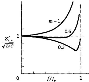
Fig. 6-10 Image impedance of  $m$ -derived half section.
