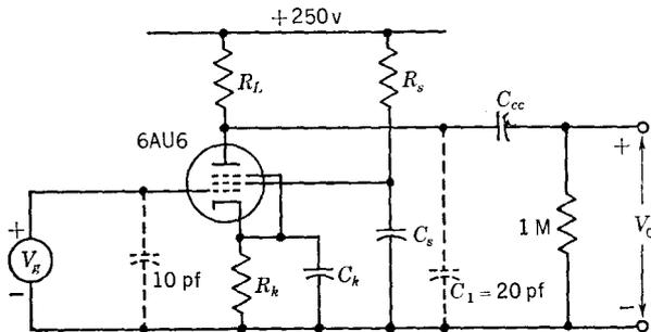
$C_1$  is the total capacitance at the plate.
