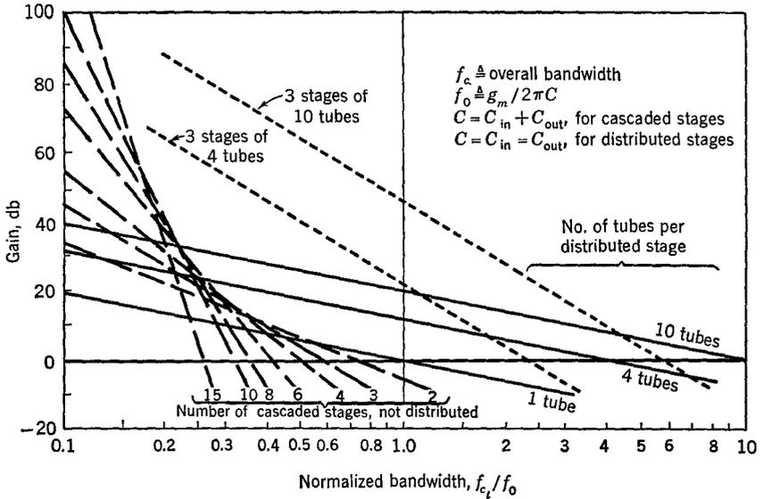
Fig. 6-16 Gain-bandwidth diagram for cascaded and distributed amplifiers.
