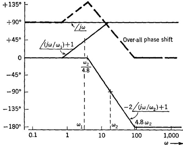
Fig. 3-9 Phase response given by Eq. (3-8d).
