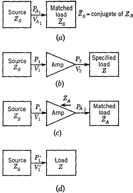
**Fig. 1-1** Gain definitions. (a) Available power from source  $\triangleq P_{A,1}$ . (b) Transducer power gain  $\triangleq P_2/P_{A,1}$ . (c) Available power gain  $\triangleq P_{A,2}/P_{A,1}$ . (d) Insertion power gain  $\triangleq P_2/P'_1$ . Two additional definitions of gain are illustrated implicitly in (b), the so-called *voltage gain*  $V_2/V_1$  and the *actual power gain*  $P_2/P_1$ . The symbol  $\triangleq$  means "defined as."
