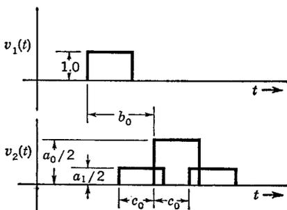
Fig. 4-35 "Paired echoes" resulting from amplitude distortion.
