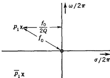
Fig. 10-3 Exact pole-zero locations for a single-tuned stage.
