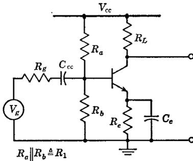
Fig. 5-2 Common-emitter stage including all sources of sag.
