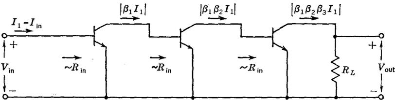
Fig. 3-17 Elementary amplifier made up of common-emitter amplifiers.
