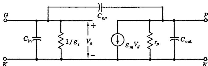
Fig. 7-1 Equivalent circuit for pentode at medium to high frequencies.
