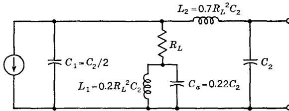
Fig. 4-9 Four-terminal "linear-phase" network for  $C_1 = C_2/2$ .
