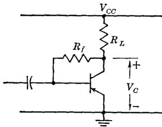
Fig. 3-26 A method of feedback biasing (cf. Fig. 3-21).
