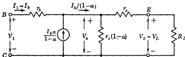
Fig. 3-18 Equivalent circuit for a common-collector (CC) stage.
