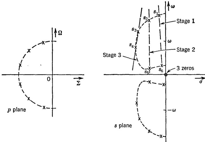
Fig. 11-10 Pole positions for the wideband case.
