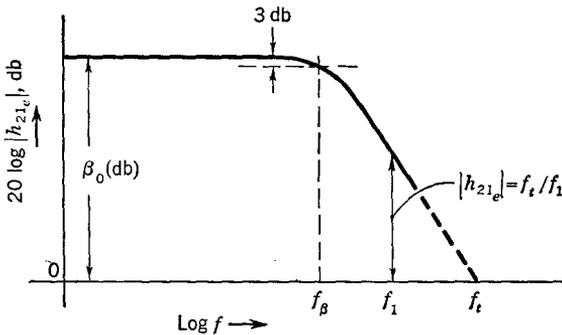
Fig. 2-25 Short-circuit current gain of a common-emitter transistor.
