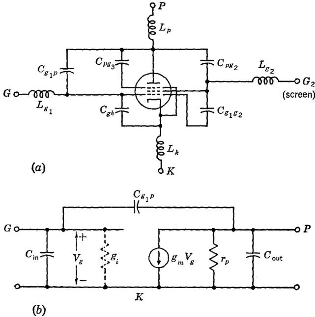
Fig. 2-15 High-frequency equivalent circuits for the pentode.
