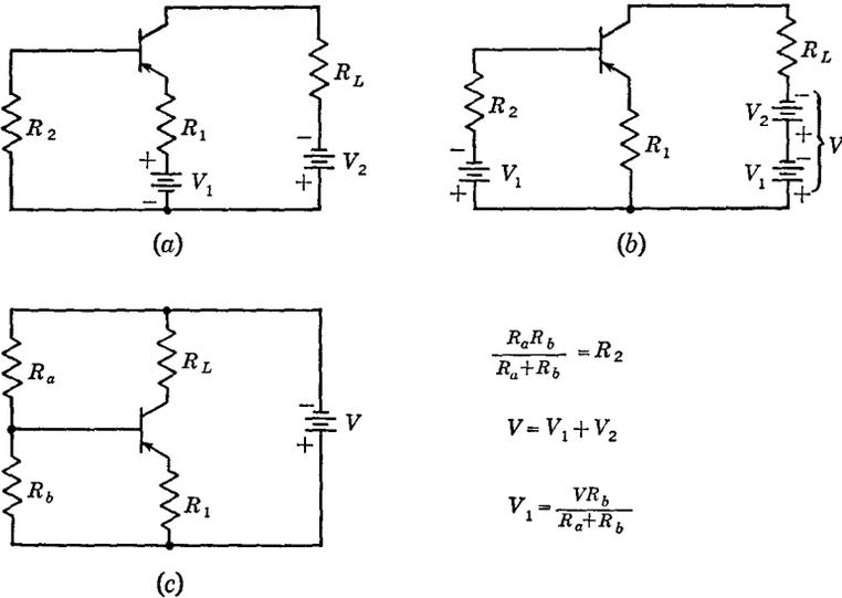
Fig. 3-25 Development of single-battery biasing from Fig. 3-23.
