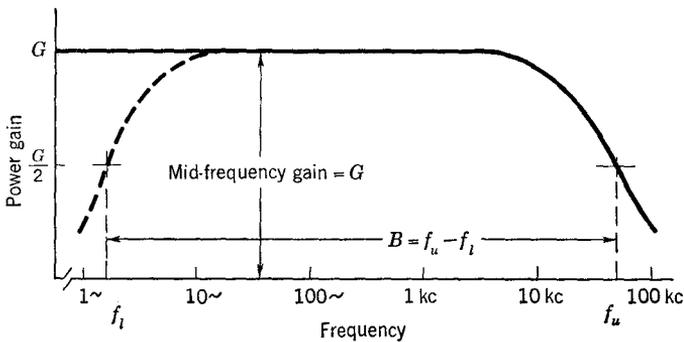
**Fig. 1-2** Typical frequency response of lowpass amplifier.
