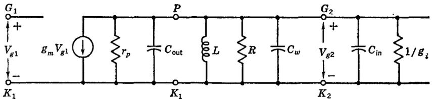
Fig. 7-2 Single-tuned interstage showing all pertinent elements.
