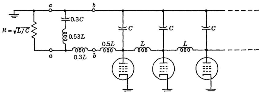
Fig. 6-11 Distributed amplifier showing the terminating half section.
