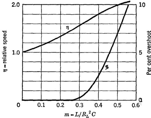
Fig. 4-3 Characteristics of a shunt-peaked stage.
