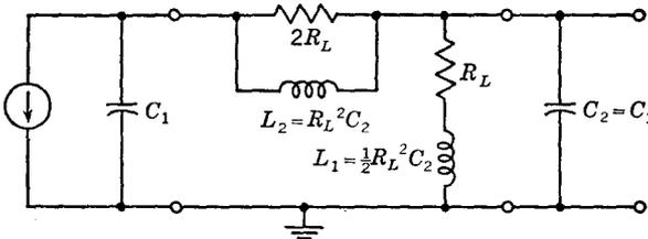
Fig. 4-10 Four-terminal network for  $C_1 = C_2$ .
